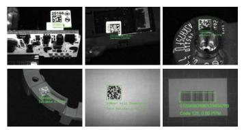
1DMax with Hotbars technology deliver high-speed reading of damaged or poorly printed 1-D barcodes as small as 0.8 pixels per module (ppm).
